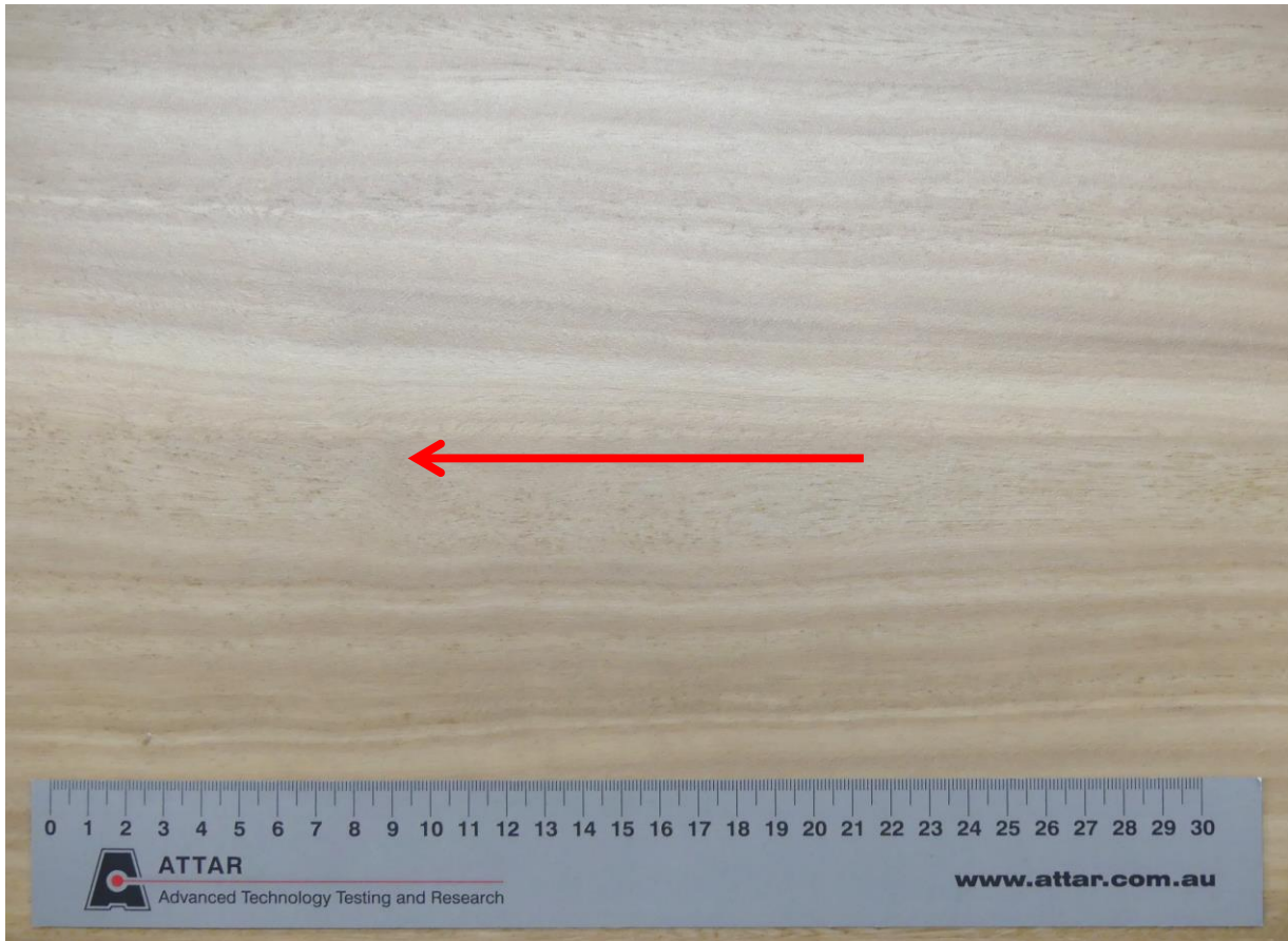
Figure 1: Bona Traffic GO Silk Matt + Bona AntiSlip applied to timber flooring Arrow indicates direction of testing
